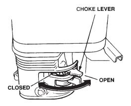
Figure 11. Choke Lever
